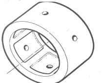
Fig: 1. Conventional Hydrostatic Journal Bearing [Ref.-1] Corresponding Author,
